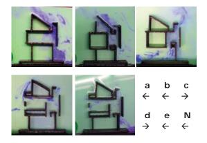
Figure 5: Flow visualization of different airflow regimes
